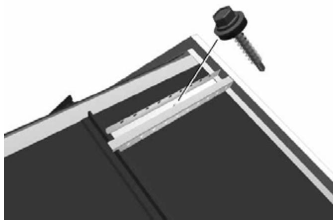
Figure 31. Fixing the Progantti ridge seal
