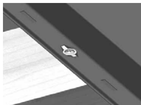
Figure 16. A screw that is too tight
