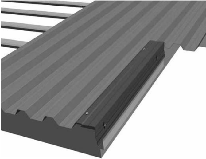
Figure 18. Installation of gable flashing
